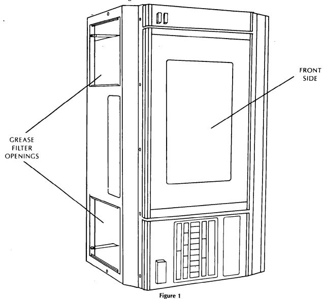
3. Remove and save two hexagonal Phillips head screws (inside grease filter openings) (Fig. 2).
